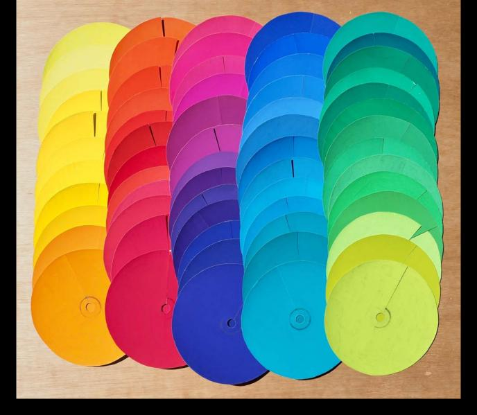
Painted discs used to find complementary pairs by partitive mixture — Pairs of discs were interleaved and spun at high speed to find combinations where the segments blended to a neutral grey.
